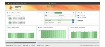
The built-in web server allows the status of the monitored batteries to be analyzed from anywhere in the network using a common web browser. The built-in SMTP mail client can be set up to send alarm messages to user-specified email addresses or text message when an alarm occurs. A rules-based system allows combinations of states/conditions to set relay contact outputs.
